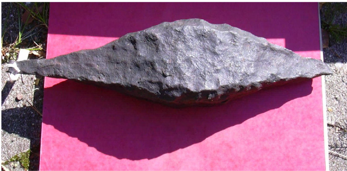
Figure 9: The lower photo shows a bar of old iron that was found in Denmark. It is about 30 cm long and 7 cm in diameter. The magnetic character of this bar was measured with the equipment shown in the upper photo. A single line of measurements was made along the length of the bar; see Figure 10 . For the measurements, the sensor of the fluxgate magnetometer moved steadily along the 1-m length of the traverse that was defined with a wooden board. The measurements were recorded in the control unit for the magnetometer, shown on the left. details
